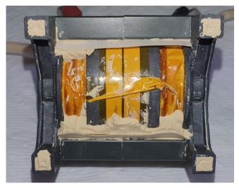
Figure 3: Ferrite Core Remained Intact
