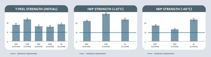
Figure 6: T-Peel and IWP strengths of typical crash-resistant structural adhesive on Cold Rolled Steel (CRS), Electro Zinc Galvanized (EZG) steel and Hot Dip Galvanized (HDG) steel and Aluminum substrates with various thicknesses
